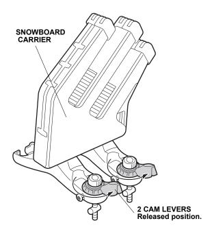
5. Attach the two bottom clamps to the top clamps.
