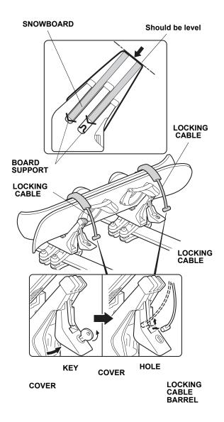
15. Check that the locking cables are installed securely, then close the covers.
