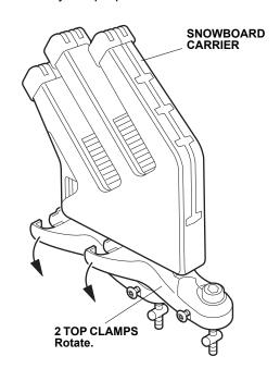
2. Install two board supports into the snowboard carrier.
